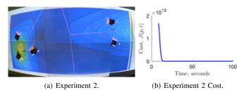
Fig. 4. Hardware-in-the-loop experiments with a team of five omnidirectional robots. (a) Final configuration for the experiment, and (b) corresponding cost over time. Similarly to the simulations, we only see one Voronoi partition here because the two Voronoi partitions overlap, since all robots have resource type k.
