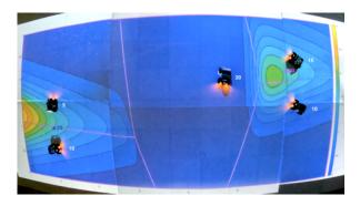
Fig. 1. Final configuration of a team of 5 robots supplying multiple resources of a single type to 2 different locations  $(\times)$ . Quantities of resources carried/demanded are printed to the right of the robot/ $\times$ . The colorbar indicates density in the space on a scale of 0 to 3, and lines represent Voronoi boundaries
