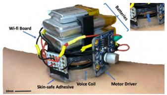
Fig. 8. Probing module with voice coil in a neutral position. The top right image shows a closer view of the voice coil, and the arrow indicates its direction of motion, which is normal to the surface of the skin. The module dimensions are 41mm × 41mm × 36mm, and weight is 87g.
